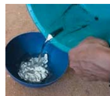
Mercury used to form gold amalgam during artisanal mining
