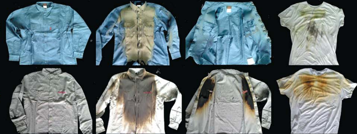
*Test performed according to IEC 61482-1-1, Method B. This test method is not used to determine Arc-Rating. Both garments passed evaluation.
