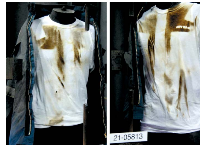
Figure 3: Fabric tested after arc exposure indicating heat transfer
