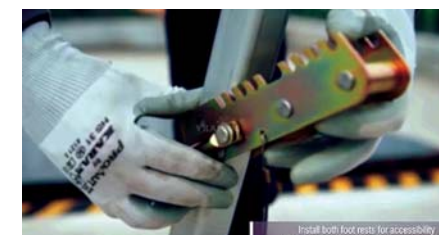
Footrests Being Installed
